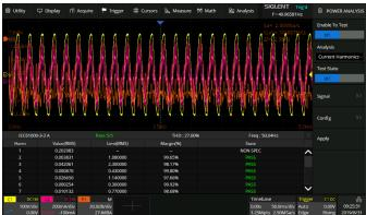
The SDS2000X Plus can control the built-in waveform generator or any stand-alone SIGLENT SDG device to scan the amplitude and phase response over frequency of passive or active circuits. The data is presented as Bode Plot. This makes it possible to replace expensive network analyzers in less demanding applications. The Power Analysis option provides a full suite of power measurements and analysis, thus improving the efficiency of measurement in switching power supplies and power device designs.
