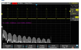
In addition to the traditional (+, -, X, /) operations, FFT, integration, differential, and square root operations are supported. The integration operation supports gating, which uses cursors to define the domain of integration
