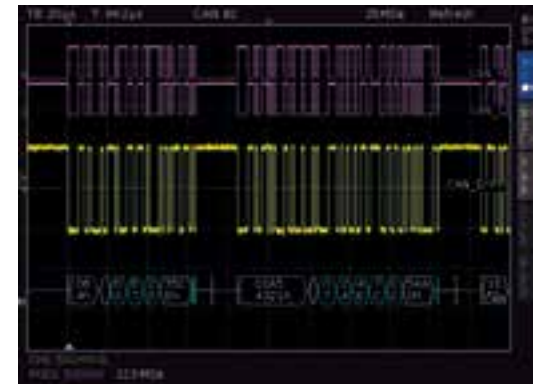
HEX decoded CAN bus signal
